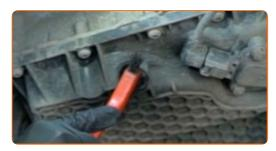
Unscrew the drain plug. Use a flat screwdriver.
