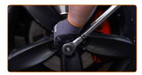
Tighten the wheel bolts using a criss-cross pattern. Use wheel impact socket #17. Use a torque wrench. Tighten it to 120 Nm torque.
