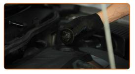
Tighten the oil filler cap.
