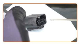
16 Attach the oxygen sensor connector.
