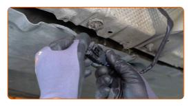
Connect the oxygen sensor wiring.
