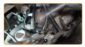
Disconnect the spark plug wires from the ignition coil.
