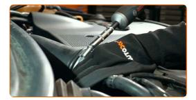
Treat the mass air flow sensor connector. Use dielectric grease.
