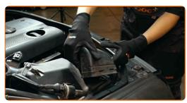
Unscrew the fasteners of the heat shield of the air filter housing. Use a Phillips screwdriver.
