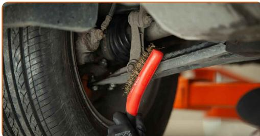
**3** Unscrew the fasteners connecting the stabiliser link to the stabiliser bar and to the suspension control arm. Use a combination spanner #16. Use a torque wrench.
