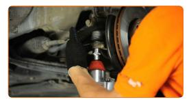
Tighten the tie rod end locknut. Use a combination spanner #21. Use a torque wrench. Tighten it to 50 nm torque.
