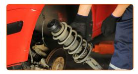
Screw the top fastening of the shock strut mount. Use a drive socket #21. Do not tighten it.
