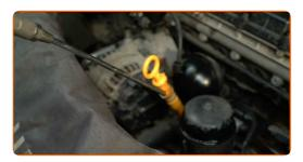
Unscrew the filter housing cap together with the old filter element. Use the 76-14F socket. Use a ratchet wrench.
