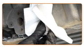
Screw in the new drainage plug and tighten it. Use a drive socket #19. Use a torque wrench. Tighten it to 28 Nm torque.
