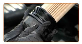
Install a new oil filter housing cover and tighten it. Use the 76-14F socket. Use a torque wrench. Tighten it to 24 Nm torque.
