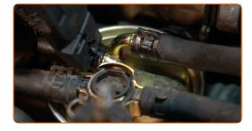
Tighten the fastening clamps of the fuel filter pipes. Use hose clamp pliers with retainer.
