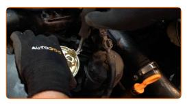
Remove the o-rings. Use a flat screwdriver.
