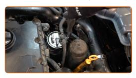
10 Remove the fuel filter pipe retainer.
