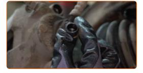
Unscrew the brake caliper fasteners. Use HEX No.H7. Use a ratchet wrench.
