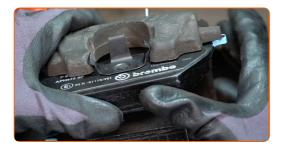
Install the brake caliper and fasten it. Use HEX No.H7. Use a ratchet wrench.
