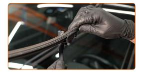
Remove the blade from the wiper arm.
