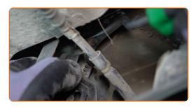
Detach the oxygen sensor connector. Use a clip removal tool.
