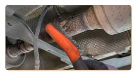
Unscrew the oxygen sensor fastener. Use a flare nut spanner #22.
