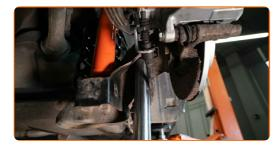
Tighten the lower fastener of the shock absorber. Important! Be sure to use new fasteners. Use a combination spanner #16. Use a drive socket #16. Use a torque wrench. Tighten it to 40 Nm torque.+90°
