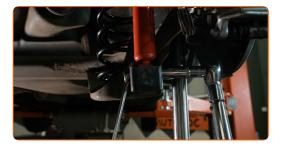
Remove the support from under the rear arm.
