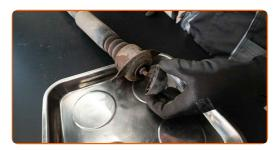
Clean the shock absorber rod fastener. Use a wire brush. Use WD-40 spray.
