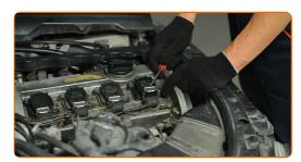
Unscrew the fasteners of the ignition coils. Use HEX No.H5. Use a ratchet wrench.
