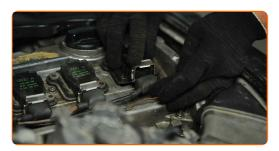
Tighten the fasteners of the ignition coils. Use HEX No.H5. Use a torque wrench. Tighten it to 12 Nm torque.
