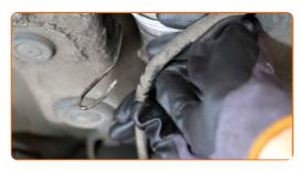
Loosen the fuel filter fasteners. Use a drive socket #7. Use a ratchet wrench.
