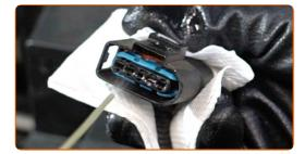
14 Attach the mass air flow sensor connector.
