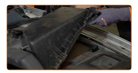
6 Cover the air intake hose with a microfibre towel to prevent dust and dirt from getting into the system.
