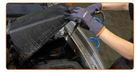
9 Insert a new filter element into the filter housing.
