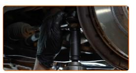
16 Tighten the tie rod end locknut. Use a combination spanner #24 (2 pieces). Use a torque wrench. Tighten it to 50 nm torque.
