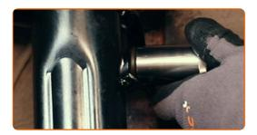
Unscrew the fastener connecting the stabilizer link to the stabilizer bar. Use a combination spanner #18. Use XZN #6. Use a ratchet wrench.
