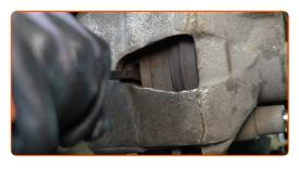
Remove the brake caliper.
