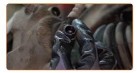
9 Unscrew the brake caliper fasteners. Use HEX No.H7. Use a ratchet wrench.
