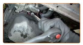
Remove the thermostat housing.
