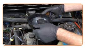
Pour coolant in the coolant reservoir.
