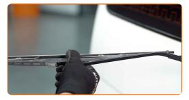
Turn the wiper blade by ninety degrees. Remove the blade from the wiper arm.
