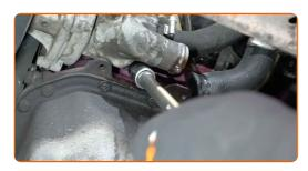
Remove the thermostat housing.
