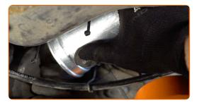
Attach the fuel filter fasteners. Use nippers.
