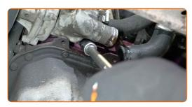
Remove the thermostat housing.
