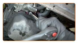
Remove the thermostat housing.
