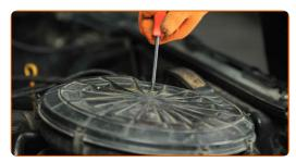
4 Release the air filter cover clips.
