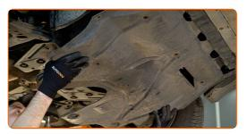
Clean the area of the oil pan drainage hole. Use a wire brush. Use all-purpose cleaning spray. 6
