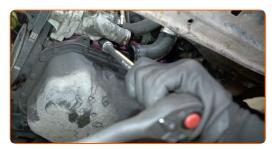
Remove the thermostat housing.
