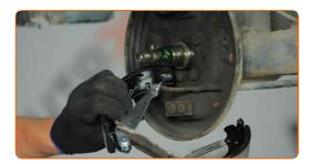
Attach the brake shoes, together with the brake adjuster, to the wheel cylinder.
