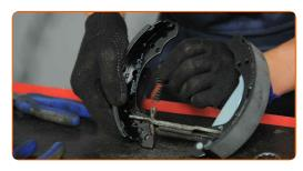
Connect the parking brake cable to the parking brake lever. Use nippers. Use pliers.
