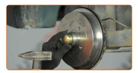
Clean the wheel rim mounting seat. Use a wire brush. Treat the surface where the wheel rim contacts the brake drum. Use copper grease.
