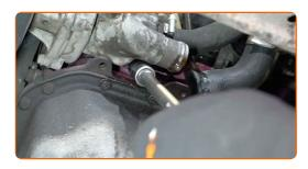
Remove the thermostat housing.
