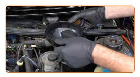
Pour coolant in the coolant reservoir.
