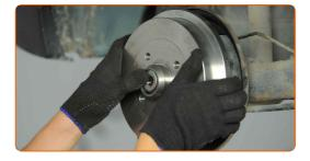
Screw in the wheel hub fastener. Use a combination spanner #24.
