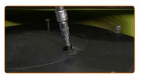
14 Tighten the fastening screws of the air filter cover. Use HEX No.H5. Use a torque wrench. Tighten it to 8 Nm torque.
