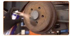
Unscrew the brake drum fastening. Use a Phillips screwdriver.
