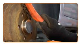
Treat the contacting surface. Use copper grease.
