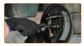
Install the retaining spring of the brake pads. Use pliers.
