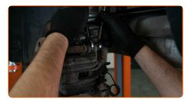
11 Remove the brake caliper.
