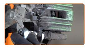
Remove the brake caliper. Use a crowbar.
