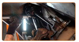
**12** Tighten the fastener connecting the stabilizer link to the stabilizer bar. Use HEX No.H5. Use a combination spanner #17. Use a torque wrench. Tighten it to 40 Nm torque.
