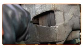
Remove the brake caliper.
