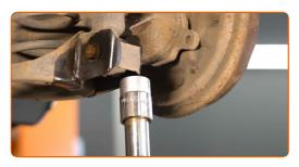
9 Remove the fastening bolt.
