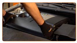
Cover the throttle body with a microfibre towel to prevent dust and dirt from getting into the system.
