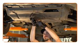
Screw in the fasteners of the lower sound insulation. Use a drive socket #12. Use a Phillips screwdriver.
