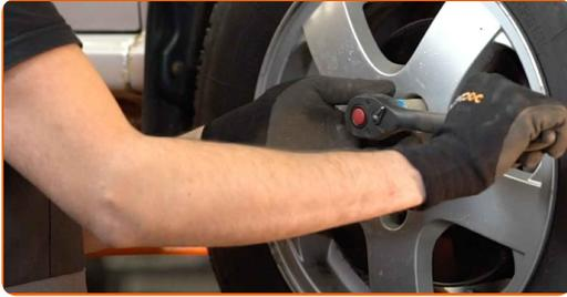
**24** Lower the car and working in a cross order, tighten the wheel bolts. Use a torque wrench. Tighten it to 120 Nm torque.
