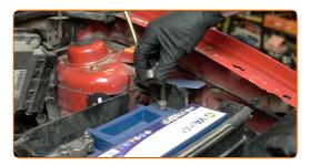
On the right side, detach the PCV valve hose from the engine cover.
