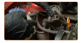
Unscrew the upper fastener of the engine mount. Use a combination spanner #16. Use a drive socket #16. Use a ratchet wrench.
