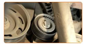
Unscrew the fastener of the serpentine belt tensioner pulley. Use a combination spanner #16.
