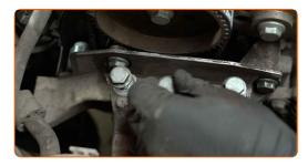
Tighten the upper fastener of the engine mount. Use a drive socket #16. Use a torque wrench. Tighten it to 50 Nm torque.
