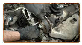
Unscrew the fasteners of the side timing cover. Use a drive socket #10. Use HEX No.H6. Use a ratchet wrench.
