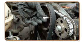
Turn the crankshaft pulley. Use 12-point socket No.21. Use a ratchet wrench.
