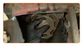
Screw in the crankshaft pulley fastener. Use 12-point socket No.21. Use a ratchet wrench.
