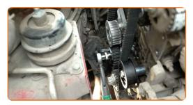
Remove the camshaft gear locking tool.
