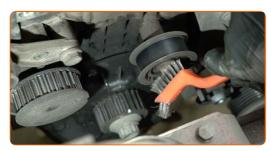
Unscrew the fastener of the timing belt idler pulley. Use a drive socket #15. Use a ratchet wrench.
