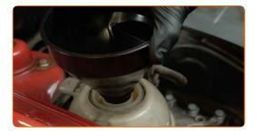
Pour coolant in the coolant reservoir.
