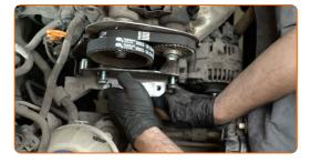
Tighten the engine mount fastening bolts. Use a drive socket #16. Use a torque wrench. Tighten it to 50 Nm torque.
