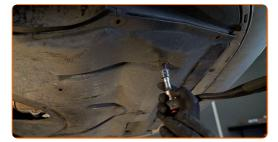
Remove the fender protection cover.
