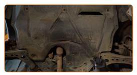
Remove the lower sound insulation.
