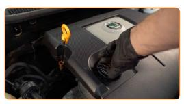
Pour oil into the engine through the filler. Required amount of oil: 3.3 l.
