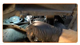
Return the tensioner pulley to its initial position.
