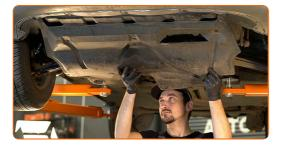
Screw in the fasteners of the lower sound insulation. Use a drive socket #12. Use a Phillips screwdriver.
