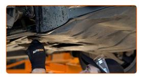
Remove the lower sound insulation.
