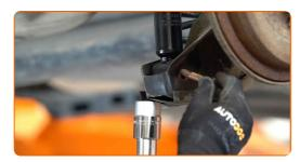
Tighten the lower fastener of the shock absorber. Use a drive socket #16. Use a combination spanner #16. Use a torque wrench. Tighten it to 40 Nm torque.+90°
